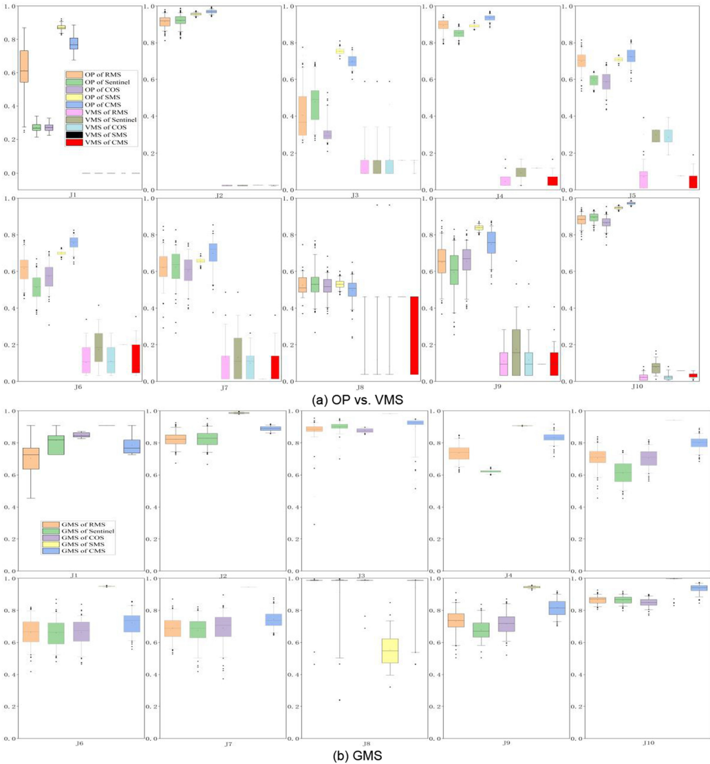
Fig. 4. The discrimination ability comparison between (a) OP, VMS and (b) GMS under a sufficient test suite for 10 programs. In (a), the legends from top to down are OP of RMS, Sentinel, COS, SMS, and CMS, VMS of RMS, Sentinel, COS, SMS, and CMS, respectively. Note that COS is skipped in J2 and J4 since there are fewer than 21 (39-18 and 109-88) mutants after filtering two mutators which means COS cannot be set to the same reduction ratio as SMS. In (b), the legends from top to down are GMS of RMS, Sentinel, COS, SMS, and CMS, respectively.
